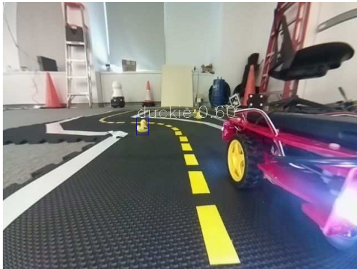
(b) Duckiebot is not detected when partially occluded and close to camera.
